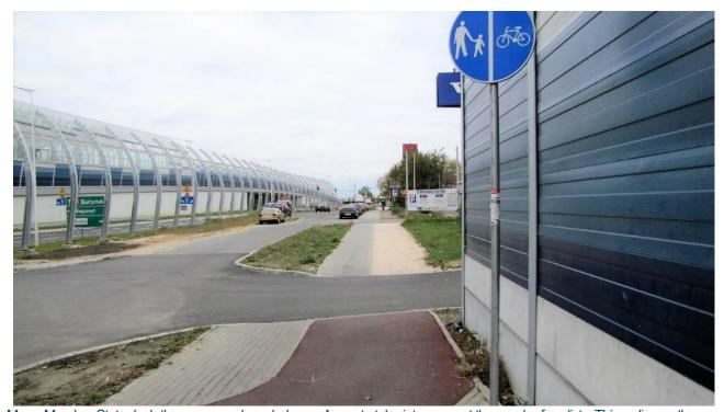
Many Member Stateslack the necessaryknowledge on **how** to take into account the needs of cyclists. This cycling path was built as a part of a TEN-Troad reconstruction project, but it is not safe to use because of lack of visibility on crossing.
