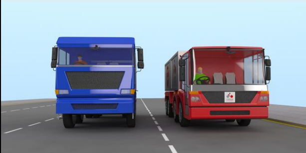
Figure 9, Comparison between a traditional construction HGV and its possible redesign with lower, better placed cab
